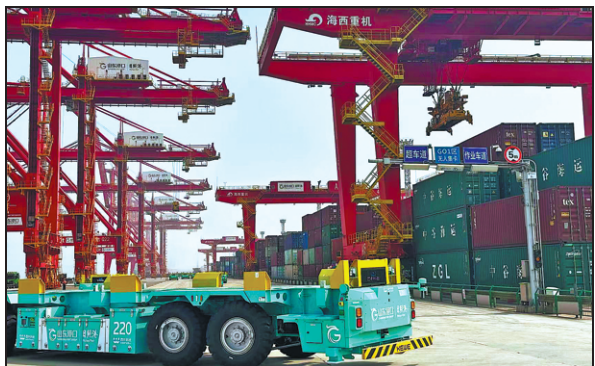
A smart guided vehicle is tested at the container field at Rizhao Port in Shandong province on Wednesday. When put into service, the vehicles will be used to shuttle containers. ZHAO RUIXUE / CHINA DAILY
