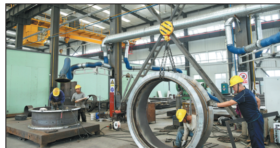
Huge gas valves are produced at a plant in Yangquan.
