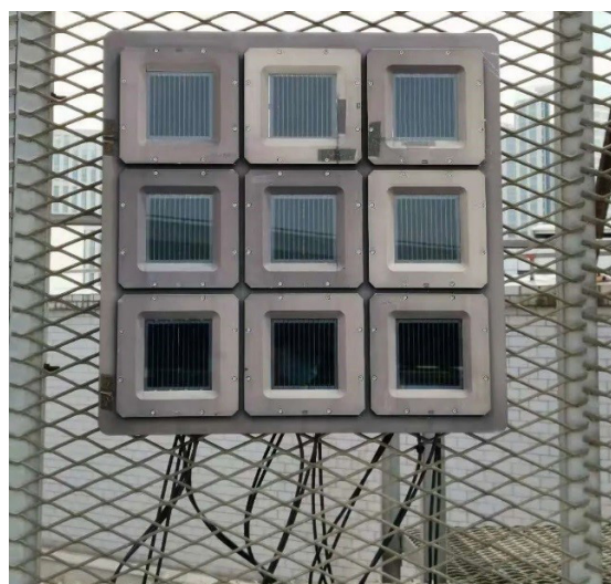
Field test system for perovskite sub-modules [IMAGE: SIC/CAS]
