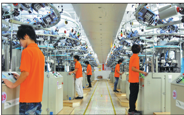
Using a computer's numerical control system, workers operate machines on the production line of a textile company in Shantou, Guangdong province. PROVIDED TO CHINA DAILY
