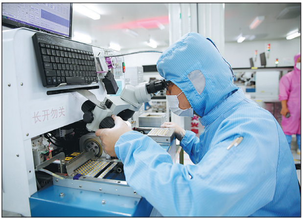
A technician works on the automatic wire bonding operation of laser at Inspur Huaguang.
