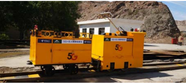
On August 24, 2020, 14 locomotives on 5 electric trams were tested at the Longshou Mine 1703 in Gansu. Unmanned driving based on 5G wireless communications is realized on all electric locomotives
