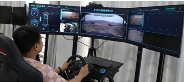
In August 2020, at the Nanshan Mine and Shangqiao Iron Mine of Masteel, dispatchers used the emergency takeover system for 5G + unmanned vehicles to remotely control the routes of unmanned mining vehicles in operation
