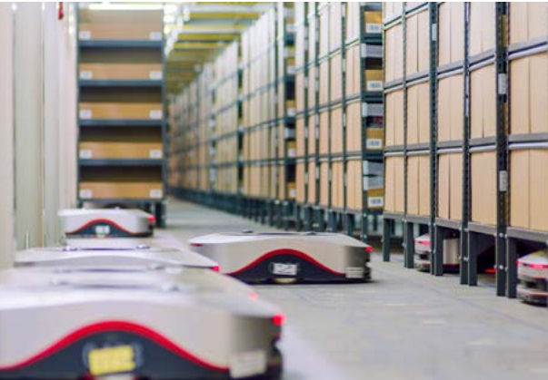
Large-scale, coordinated AGV operation supported by China Telecom's private 5G network. The picture shows AGVs in operation
