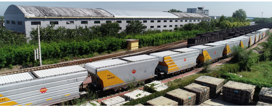
Green transportation: Integrated with multiple new technologies such as the light-weight aluminum alloy body, environment-friendly movable top cover, self-discharging bottom door opening and closing in two directions, coupler buffer with long overhaul period and integrated braking system, and with the technical characteristics such as environmental protection, heavy load and efficiency, KM81 Coal Hopper Car of Railway Equipment Company can guarantee the vehicle application safety to the maximum extent and assist the “comprehensive blossom” of economic benefit, social benefit and environmental benefit.
