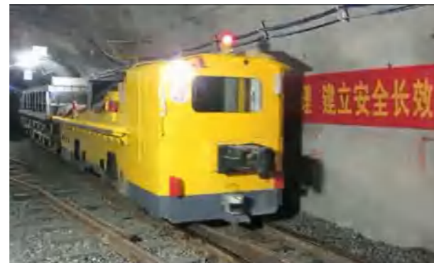
▲ Unmanned electric locomotive underground the mine
