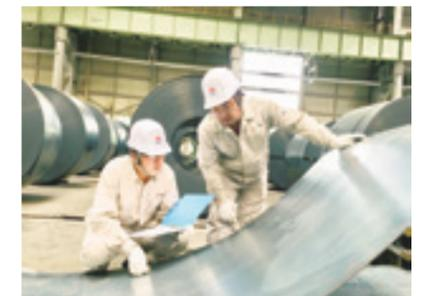
Checking the quality of steel plate surface
