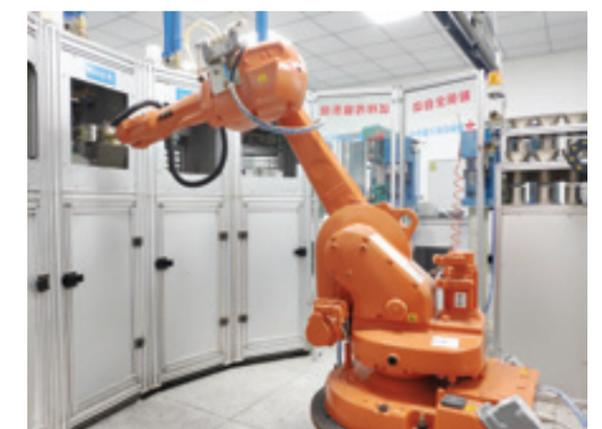
The "robot" takes out the molten steel sample from the sampling cabinet
