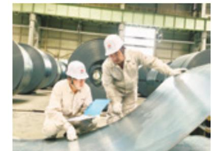
Checking the quality of steel plate surface
