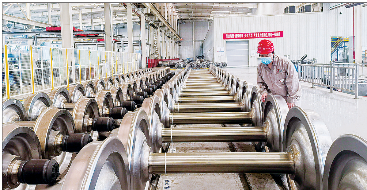
A worker inspects the quality of train wheels produced by the rail transit equipment unit of Taiyuan Heavy Industry. WANG PEI / FOR CHINA DAILY
