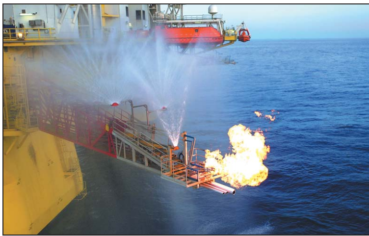
A drilling platform is extracting methane gas trapped in icelike crystals in the seabed of the South China Sea. Tests are being done for future commercial use. PHOTO PROVIDED BY CHINA GEOLOGICAL SURVEY
