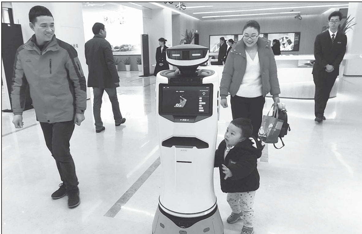
A child is attracted by robot Xiaotu at a public service center in the Xiaoshan district of Hangzhou, Zhejiang province, on Wednesday. The robot can issue numbers for waiting, provide simple public service guidance and recharge a mobile device. The center opened on Wednesday, enabling residents and companies to complete administrative procedures in one run by integrating government resources. LONG WEI / FOR CHINA DAILY
