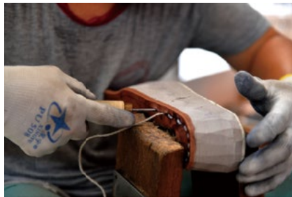
Making thick boots needs broach and twine.
