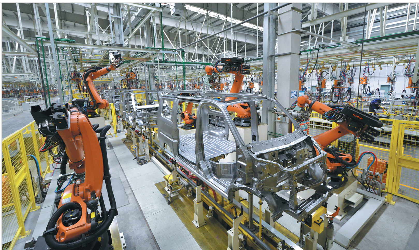
Fully automated robots weld the bodies of automobiles in a workshop in the Foton Shandong Multifunction Plant in the Weifang Hi-tech Industrial Development Zone.
