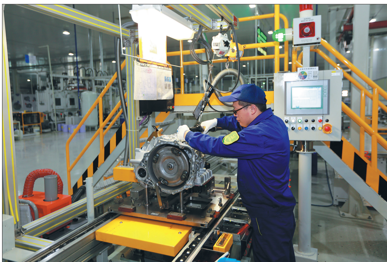
A technician at Shengrui Transmission assembles one of the company's front-engine, front-drive 8-gear auto transmissions.
