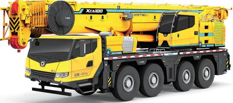
including a double boom pin and singlecylinder pining telescopic system, an independent suspension system with large load and single beam and intelligent crane boom. It has more powerful lifting and driving performance compared with its counterparts around the world.
