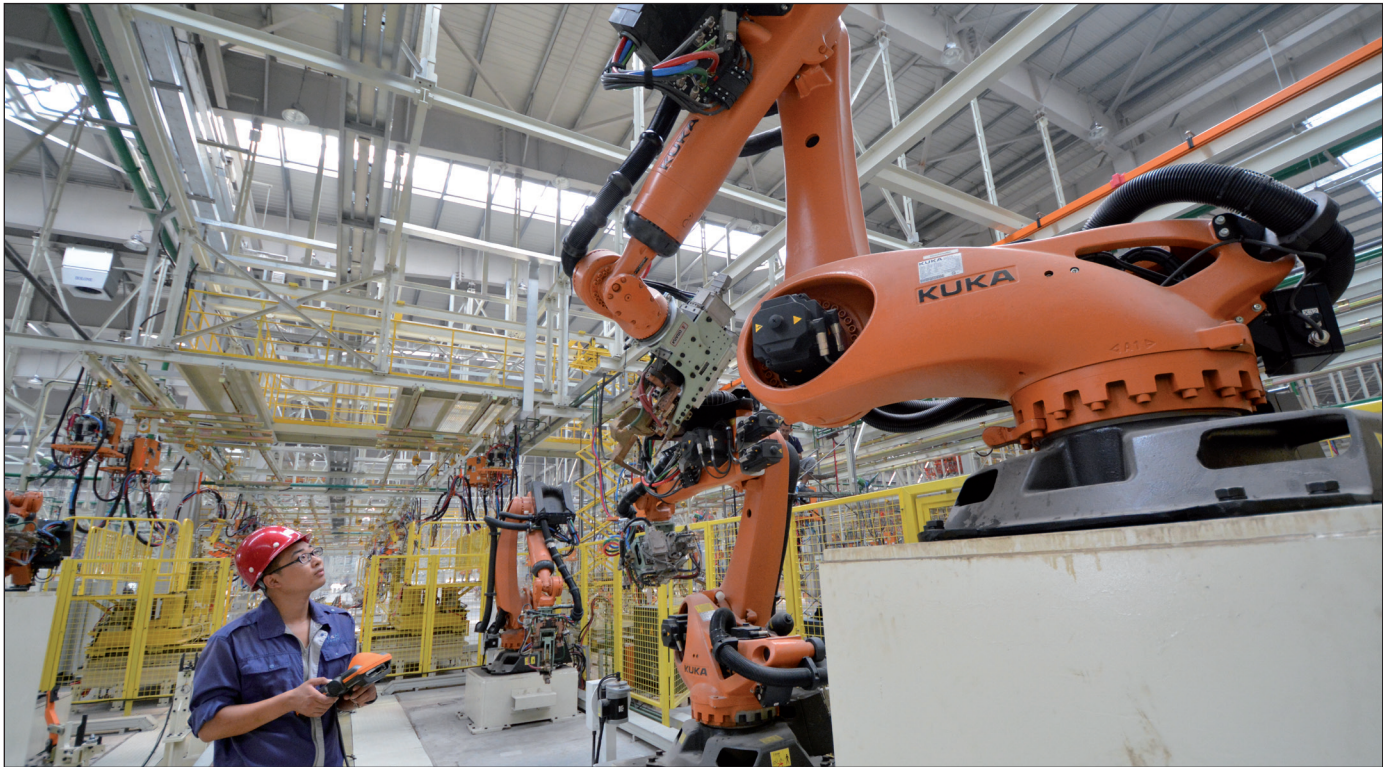
A worker operates a welding robot at the Foton Shandong Multifunction Plant.
