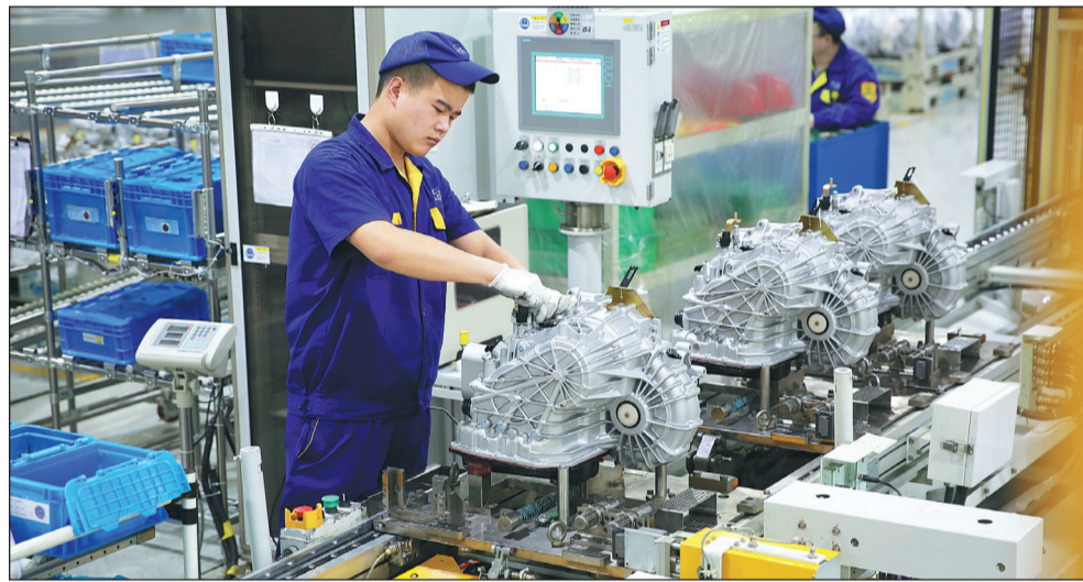
A technician with Shengrui Transmission Co assembles an 8-gear automatic transmission at the company's production line.
