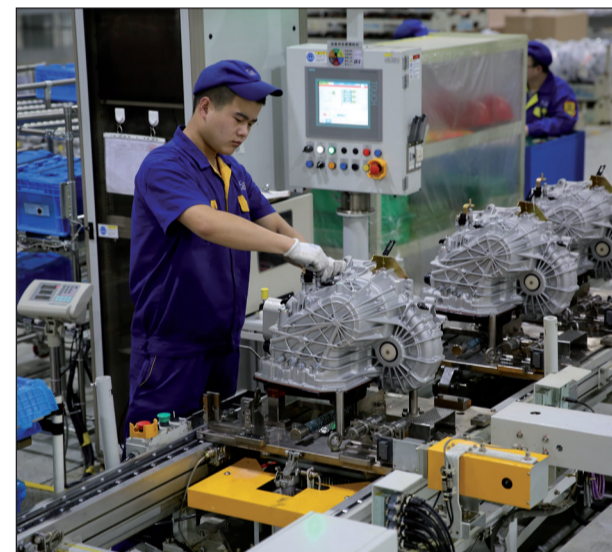
A technician at Shengrui Transmission Corp assembles 8AT units on the company's production line.
