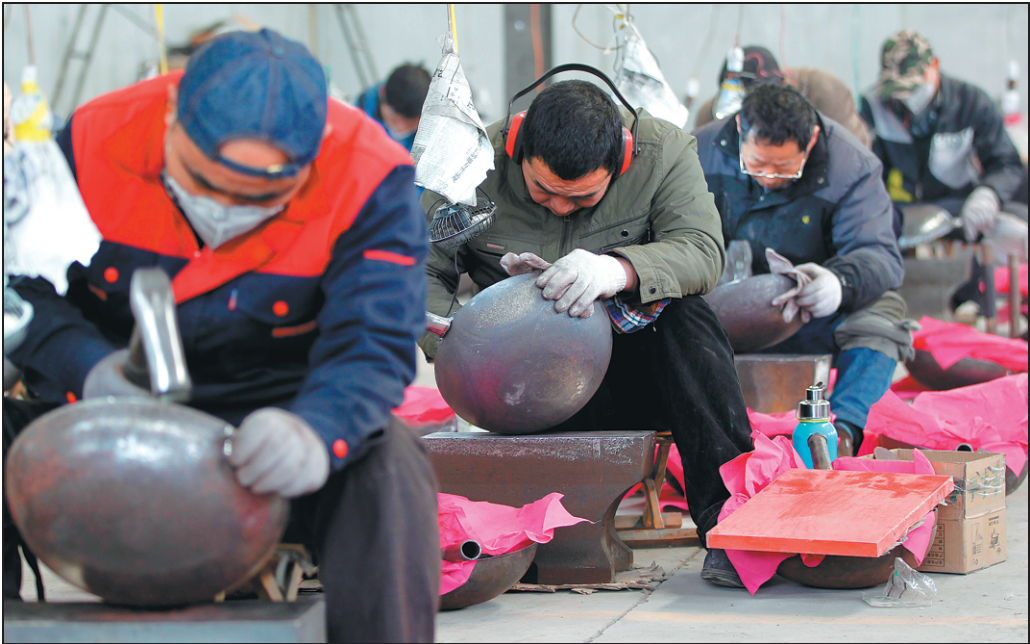
Craftsmen hammer out iron woks on Wednesday in Zhangqiu district, Jinan, Shandong province. The woks, which have boomed in popularity since they were featured on the TV show A Bite of China last month, are made using 12 steps. CHEN ZEBING / CHINA DAILY
