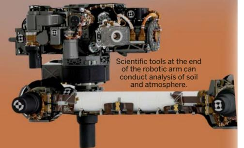
Scientific tools at the end of the robotic arm can conduct analysis of soil and atmosphere.
